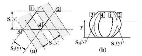
Fig. 15 - (a) A case where  $S_3(y)$  is compatible with S1(y) and  $S_2(y)$  in a horizontal plane. (b) The condition for the compatibility of the whole silhouettes.
