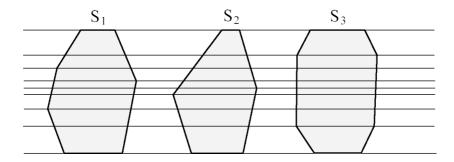
Fig. 24 – Dividing polygonal silhouettes into strips
