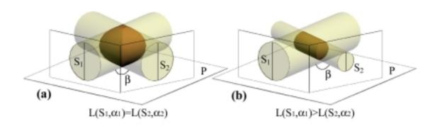
Fig. 7 - In (a) it is shown how to find an object compatible with two silhouettes having two equal 1D projections. If this condition is not satisfied, the silhouettes are not compatible (b).
